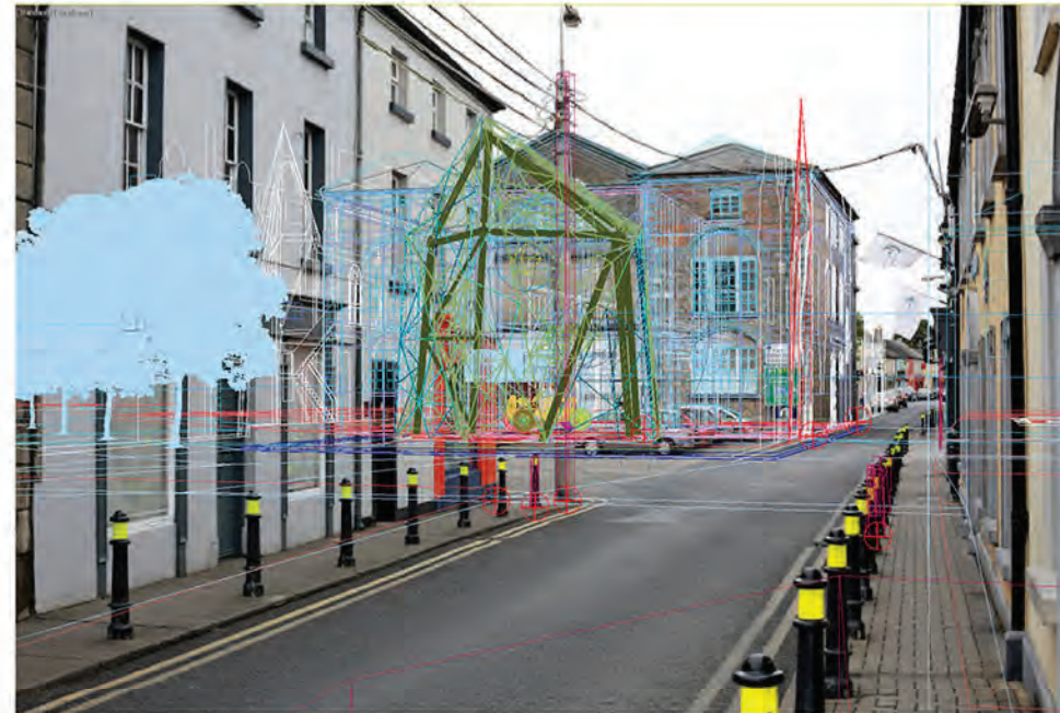
Example screen grab from the 3d software showing the existing building modelled with the surveyed reference points marked in red overlaid and matched to the photograph.
